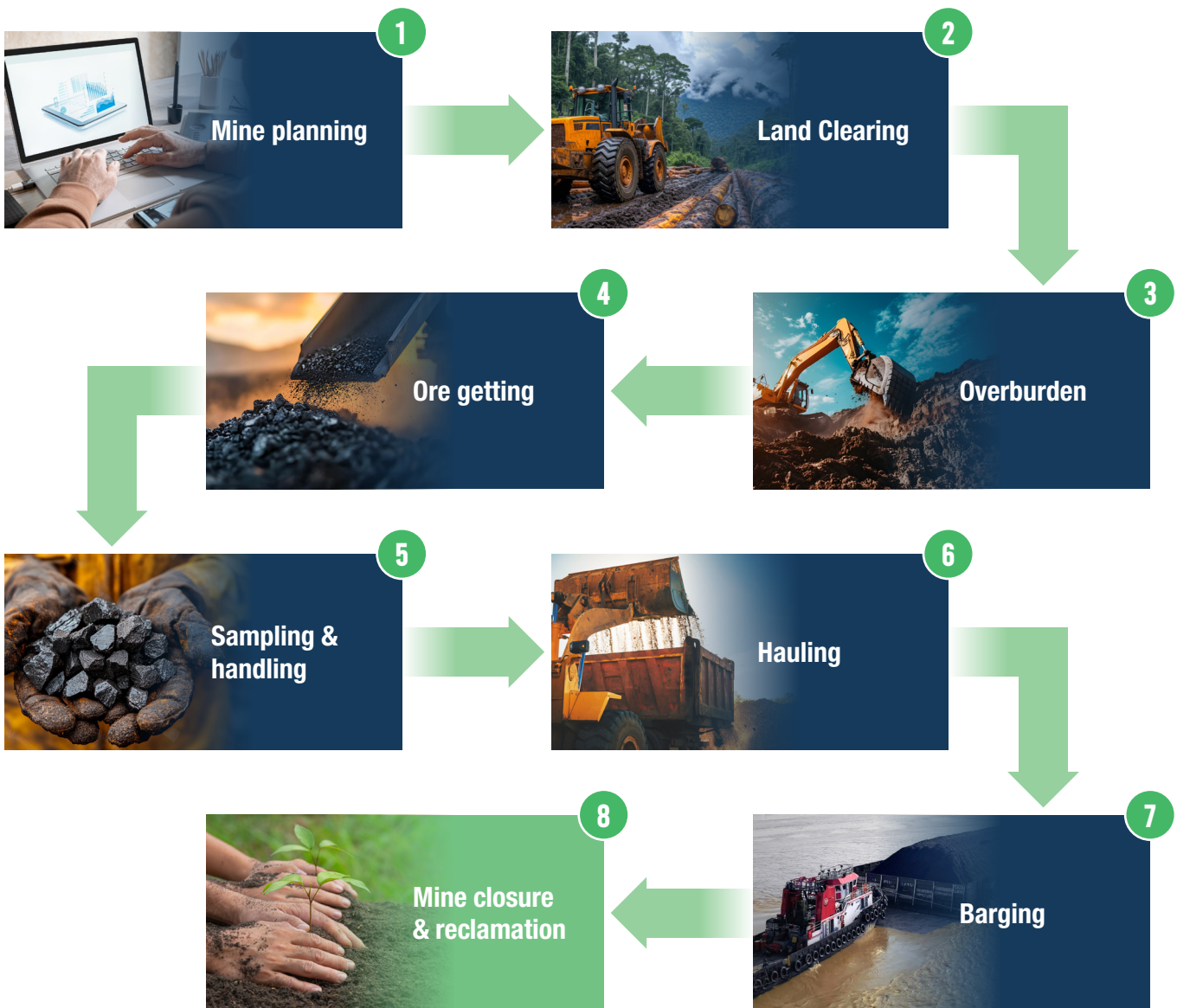
Figure 25. Stages of laterite nickel ore mining activities
